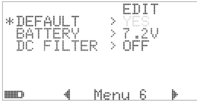
Figure 4-30 Resetting to default factory settings
